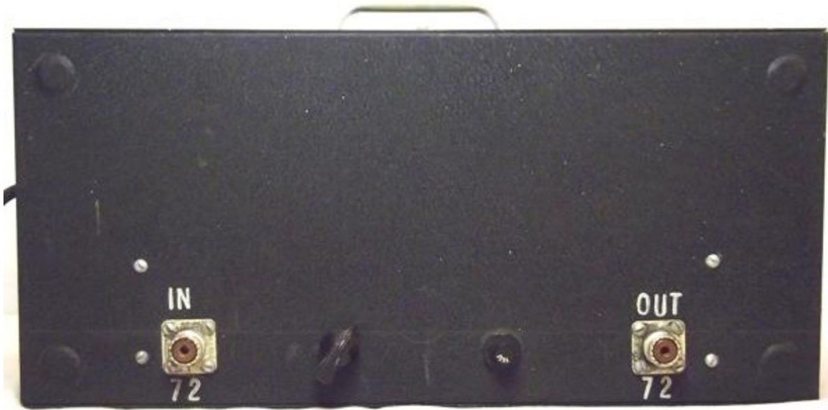
Figure 3. Jerrold CA-6 MATV Channel Amplifier Rear Panel Showing 72-Ohm Coaxial I/O (Chandler, 2019)
